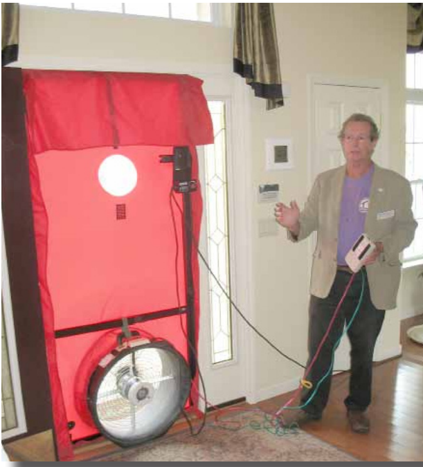
HERS rater Frazer Dougherty demonstrates how a blower door is used to measure the airtightness. The ENERGY STAR Homes Law requires a HERS rating of at least 84 before a CO is issued.
